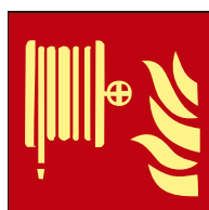
Ref. 11 Boca de incendio
